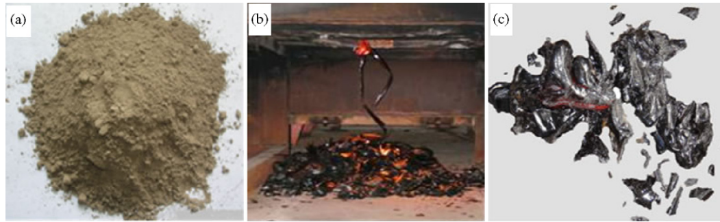
Fig. 2. Appearance of fly ash before and after vitrification: (a) raw fly ash before vitrification, (b) discharging molten slag after vitrification, and (c) cooled molten slag.
